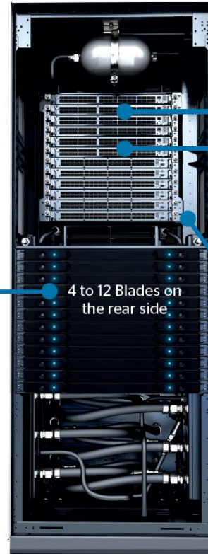
42U cabinet rear view
