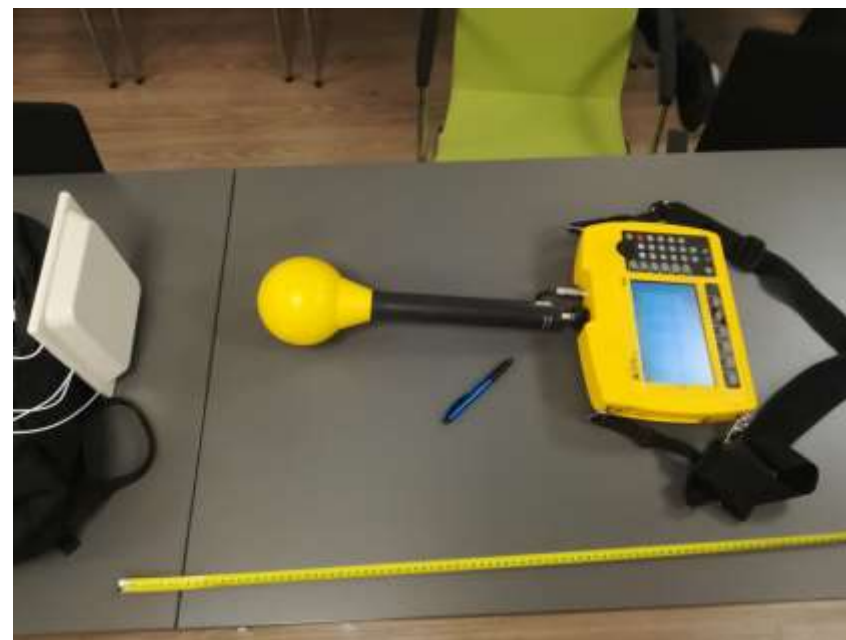
Spektralni analizator Narda SRM 3006 in 3D antena Narda 3502
